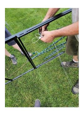
STEP 4: Assemble the top of the Manger Structure. NOTE: You will need Qty. 2 3/8" nuts to complete this (there are bolts welded on to the Manger Structure pieces
